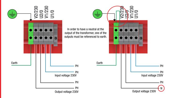
The input power supply shall be provided at terminals U1 and V1.
